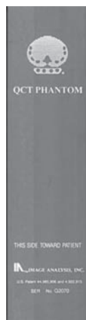
FIGURE 20-23 The long axis of the calibration phantom is placed on and parallel to the long axis of the scanning table, under the patient’s torso. Photo courtesy of Image Analysis, Inc.
